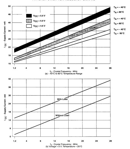
Figure 4. Typical CMOS  $I_{CC}$  vs Frequency
