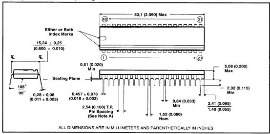
NOTE A: Each pin centerline is located within 0,254 (0.010) of its true longitudinal position.
