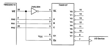
Figure 3. I/O Decode Circuit
