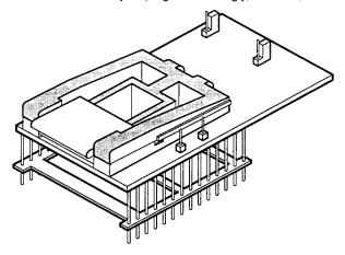
Figure 5. EPROM Adapter Socket
